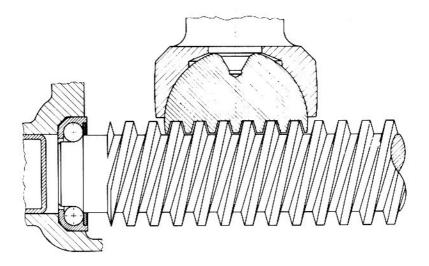
The steering gear set consists of steering worm, sector and sector shaft.
