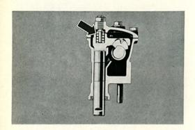
5/340 This picture shows the operation. The pin and spring, shown by the arrow, play a very important part. If the spring pressure is too high or too low, or if the length of the parts deviates from the correct measurements, incorrect play can result between worm, sector and sector shaft even with the adjusting screw properly set.
