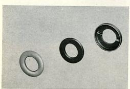
5/120 The thrust bearing, installed between the steering knuckle and the torsion arm link, consists of a thrust washer, plastic washer and a cover. Here you see the cover with two different synthetic washers which have been installed intermittently. The dark one should always be used during repairs instead of the lighter colored one. If the old washer shows no signs of wear it is better to reuse it as a new one can settle slightly during use.
