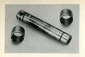
5/40 The king pins and bushes are removed in the Repair Press. If king pins and bushes are badly worn as shown in this picture, they should be replaced. Before installing them the front suspension should be thoroughly checked.
