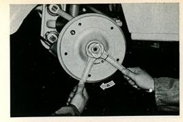
5/220 In this way the bearing play can be correctly adjusted. The bearings are correctly adjusted if the thrust washer can just be moved by a screwdriver. After installing the wheels check front axle tread and rectify if necessary.
