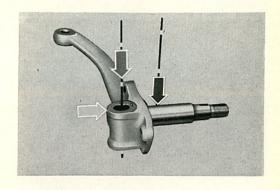
5/90 After checking and measuring, the king pin bushes are pressed into the torsion arm link on the Repair Press. Always press the bushes towards the outside of the torsion arm link as shown by the arrow.
