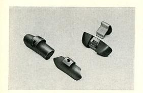
5/460 There are various sizes and types of weights. Only weights with short retaining tongues — as shown below — may be used for turbeless tires as otherwise the seating between tire and rim can be affected. The weight with the long tongue — to the left of it — can only be used for tires with tubes. At the top right you see a third weight which is in two parts, is easy to fit and ensures a perfect seat of the tubeless tire and a tight fit on the rim.
