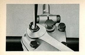
5/330 After installing the thrust spring and pin and tightening the cover, adjust the radial play. Tighten the adjusting screw as far as it will go and then back off approximately 1/8 of a turn i. e. 45°. Hold the adjusting screw in this position and tighten the lock nut. On all accounts back off as prescribed to ensure that the correct play between thrust pin and sector shaft is obtained.
