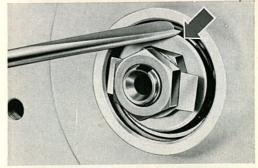
5/230 If the steering is heavy and does not self-center the oil level in the steering gear should be checked first. The wheels are then locked to the right so that the sector and sector shaft arm are at the lower end of the worm.
