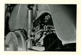
5/380 Check tie rod ends for wear as any play here encourages kick and shimmy. This is done by holding the tie rods close to the ends and attempting to move them up and down as shown by the dual arrow. If the ball joints show signs of play. the tie rod or tie rod end has to be replaced.
