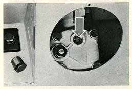
5/240 The oil level is correct if the root of the worm thread is just covered with oil as shown here. Then check the steering gear adjustment and rectify if necessary. If the steering trouble still exists, the steering gear must be removed and all components carefully examined.
