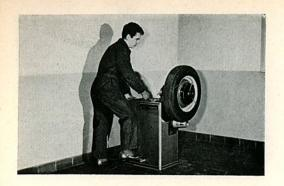
5/450 Finally check the wheels and tires. The maximum radial and lateral run-out must not exceed 1.5 mm. Any unbalance of wheels and tires is determined by a wheel balancer. The result shows the location and the weight required to balance the wheels.
