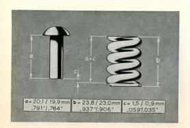
5/350 The spring pressure should be between 60 and 75 kg (132—165 lbs.), and if it is too high the sector will be pressed too hard on the worm and will cause heavy steering. In this case the spring can be shortened by grinding. Measure the length of the pin shaft a and the free length of the spring b. The correct measurements are shown on the picture. The spring can be ground down until it is still 1.5 to 0.9 mm longer than the pin shaft, measurement c. The length of the spring is a + c.
