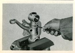
5/130 When assembling steering knuckle, thrust bearing and torsion arm link there should be no end-play. This factor is of great importance in cases of kick and shimmy. First of all take the thinnest thrust washer 3.56 mm when installing the thrust bearing and then measure the end-play with a feeler gauge. In this case it is 0.15 mm and the assembly should take place with a preload of 0.05 ± 0.02 mm.
