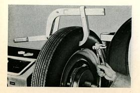
5/470 Here you see the tire walls being pressed in with a clamp and the weight being attached. Take care that the tongue is not bent back too far when installing, as otherwise the weight may work loose when driving.
