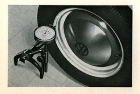
5/410 Mark the tires with chalk at the point of contact. Set the gauge dial to zero, remove the gauge and push the car forward by half a wheel turn.
