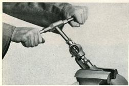
5/110 The bushes are now reamed up to the correct dia. 18.034—18.016 mm with an adjustable reamer. The bushes must be free from scores and chatter marks. There is a danger when reaming split bronze bushes that the reamer will get blunt quicker.
