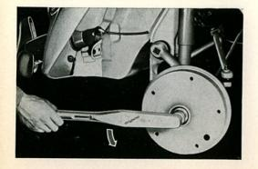
5/200 After installing the brake drum adjust the front wheel bearings. The picture shows how this can be done if a torque wrench suitable for 4 mkg (29 ft. lbs.) with a 27 mm socket is available. First tighten the inner nut to 4 mkg (29 ft. lbs.), then fit a new lock plate and loosely screw on outer nut.
