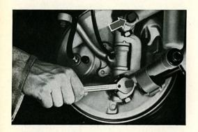
5/190 The torsion arm link pins should be carefully adjusted as follows: Fully tighten the torsion arm link pins and then back off 1/8 of a turn. Then retighten the link pins until the first resistance is felt.
