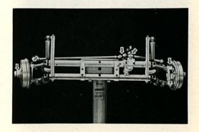
5/30 First of all try to counteract this stiffness by greasing. To do so, lift the car so that the front axle is unloaded. While greasing turn the torsion arm link pin to and fro to ensure that the new grease can penetrate better. If this measure has no result the steering knuckle and torsion arm link are to be removed and disassembled.
