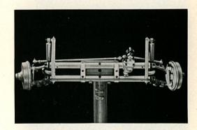
5/20 The picture shows a complete front axle. All parts shown with arrows can cause steering troubles, such as heavy steering, kick and shimmy and noises or encourage such faults. If the steering is hard to turn for example, the cause may be king pin binding. This can easily be determined by removing the tie rod from the steering knuckle arm and moving the wheel to and fro. The various causes for stiffness at this point call for a careful check of the front suspension.
