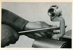
5/100 The cover is held in position at the top of the torsion arm link to prevent rotation. If new bushes have been installed, the upper bush has to filed in accordance with the grooves in the steering knuckle. Remove all filings carefully.
