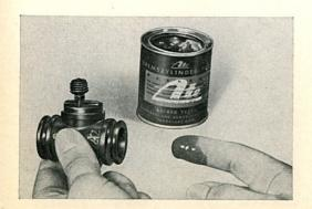
2/220 The brake lines should be flushed with brake fluid only. Dirty brake fluid should be replaced by fresh fluid. As only the sealing lips of the cup come into contact with brake fluid in actual operation, pistons and cylinder interiors should be lubricated with brake cylinder paste. This lubricant has no affect on rubber and helps to prevent corrosion.
