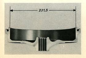
2/330 Brake drums which are grooved or badly worn can be turned out up to a diameter of 231.5 mm. Always ensure that a minimum wall thickness of 4 mm remains.
