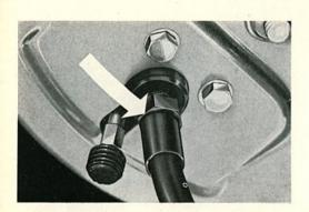
2/260 When tightening brake line and hose unions there is a tendency to use excessive force. A tightening torque of 10—18 ft. Ibs is really quite sufficient. If this torque is exceeded there is a danger of breaking the threaded adaptor or damaging the seat for the nipple. The importance of details of this type will be realised if we consider that pressures of up to 1400 psi are reached when the brakes are applied.
