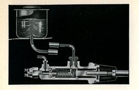
2/80 Excessive heat in the brake drums transfers to the brake fluid which then expands and causes the pressure in the brake lines to rise. To prevent this pressure rise from leading to dragging of the brakes, the check valve releases and allows the pressure to equalize to the reservoir via the by-pass port. This operation shows how important it is to ensure that the by-pass port is not blocked.
