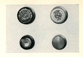
2/120 This is done by first measuring the piston diameter with a micrometer. As the piston may not be quite round, measure it at several places.
