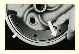
2/360 Excessive taper in the drum and distorted brake shoes or backplates can be the cause of the trouble if the lining only touches at the point shown here by arrow B. As a result, the brake shoe moves in the direction shown by arrow A when the brakes are applied. When the brakes are released the brake shoe moves back, hits the backplate and causes a knocking noise.
