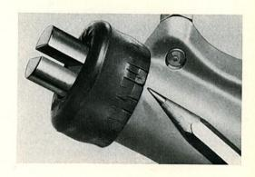
2/240 This is not a picture of an excavation find dating back to early Roman times, but a very much enlarged view of a rusty brake line. The effects of weathering over a period of several years service can make this brake line just as dangerous as a pipe which is badly chafed, kinked or flattened by stone damage.
