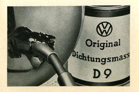
2/390 To prevent water from entering the brake drum, the slot between backplate and brake cable retainer should be sealed carefully with VW D 9 sealing compound.
