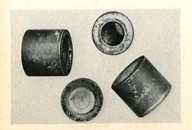
2/160 A glance at these corroded pistons shows what happens if alkaline solutions get into the wheel cylinder when cleaning dirty backplates or spraying axles after removal. 2/170 Here two cups which have been damaged by seizure marks in the cylinder are compared with a good cup. Before these parts are replaced it is advisable to have a good look at the cylinder to which they belong.
