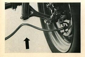
2/270 Make sure that the brake hoses on the passenger car do not hang down and affect the ground clearance. To give the hoses a slight curve to the front as shown here, twist them from about 90° to a maximum of 180° before securing them at the frame end. Great care must be exercised when greasing, spraying or painting the vehicle as the hoses are not paint or oil resistant.
