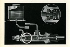
2/40 When the pedal is released, the tension of the brake shoe return springs forces the fluid back to the master cylinder where it lifts the check valve from its seat and passes into the pressure chamber. Whereas the piston returns to its original position very quickly when the pedal is released, the fluid flows comparatively slowly. This can create a vacuum in front of the main cup for a short time.
