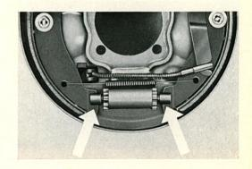
2/300 One essential feature for uniform, effective braking is the coefficient of friction of the brake linings. When fitting new linings, always ensure that at least the two wheels on one axle are fitted with linings which have the same coefficient of friction. Oiled-up linings cannot possibly fulfill this requirement.
