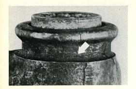
2/150 At the opposite end of the scale are sticking pistons. Even if the damage is not so serious as in this picture, the cylinder, pistons and cups should be replaced without hesitation.
