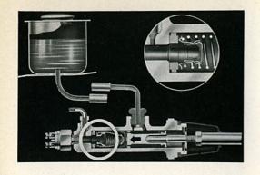
2/30 When the brake pedal is depressed, the piston forces the brake fluid past the check valve along the brake lines to the wheel cylinders. An enlarged view of the check valve on the right shows the rubber cap which opens and closes the system.
