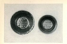
2/200 All the other rubber parts in the hydraulic brake system are equally susceptible to damage from mineral oils. This picture shows a cup which is swollen due to the influence of mineral oil compared with a good cup.
