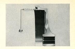
2/350 If one end of a brake shoe with a normal lining is pressed against the friction surface of an oversize drum as shown here, there will be a steadily increasing gap towards the other end between drum wall and lining. This gap is proof that reworked drums should only be used together with oversized linings. This is the only way to ensure that the lining contacts the brake drum over the full area.
