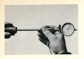
2/140 When the inside measuring gauge is inserted into the cylinder, the clearance can be read off on the dial indicator as the variation from zero. This clearance must not exceed 0.26 mm (.10"). Parts which are getting near to this limit should be replaced to be on the safe side. The presence of burrs on the backplate or on the cylinder contact surface can cause cylinder distortion. For this reason the inside measuring gauge should be turned when taking the reading.
