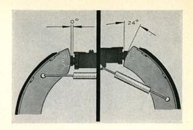
2/290 The brake shoes can move freely in the slots in the piston ends and the adjusting screws and are thus self centering. This more or less eliminates the tendency to brake grabbing. To further the self-centering properties, the sliding surfaces are lubricated with high melting point graphite grease on assembly.
