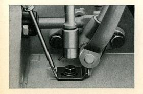
2/100 The proper way to adjust the play between push rod and piston is by means of the elongated hole in the brake pedal stop bracket. To prevent the bracket from moving in service, ensure that there is always a galvanized spring washer on the securing screw.
