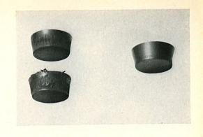
2/180 As the pistons should be a suction fit in the cylinder, any cylinder showing signs of rust like this one, is not fit for further use. Reworking with emery cloth or grinding paste is not satisfactory from a technical or safety point of view.
