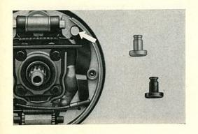
2/380 Moisture which occasionally enters the brake drum can cause the pin for the lever of the handbrake linkage to seize. When this happens, the brakes stay on when the handbrake is released. In such cases it is advisable to fit a galvanized pin and not to just free the linkage off.
