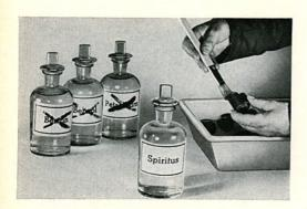
2/210 This is why the rubber parts and other parts of the cylinders should never be washed in gasoline, benzine or kerosene. Apart from brake fluid itself, the only other liquid to be used is methylated spirits. After cleaning with meths, the parts must be dried thoroughly.
