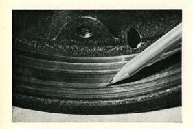
2/320 Before new or newly lined brake shoes are installed, the drums must be checked for grooving and radial and axial run-out. All friction surface damage reduces the efficiency of the brakes and thus minimises the success of the entire repair operation.
