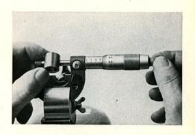
2/130 When the measurement has been taken, set the inside measuring gauge to the micrometer reading without altering the micrometer and then zero the dial indicator.
