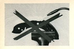
2/310 This is one very poor way of trying to make oily linings fit for use again. Burning off, boiling or washing oiled-up linings is not only useless, it also endangers the safety of the vehicle.
