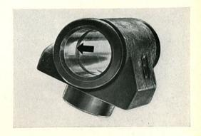
2/190 One of the main causes of such corrosion is damaged protective boots. Apart from the fact that these boots are often loose, aged or torn they can be softened in a very short time by grease escaping from overfilled wheel bearings.
