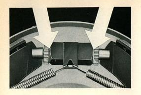
2/370 On older vehicles, knocking noises at the wheels can be caused by the fact that the contact faces of the nuts have worn into the anchor block. The edge thus formed on the nut slips on the end face of the anchor block when the brakes are released and causes a knocking noise. This trouble can be eliminated by fitting a washer between the anchor block and the adjusting nut on each side.
