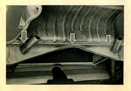
14/34 It is not always possible to make the metal sheets which lay within the spray range of the front wheels watertight.
