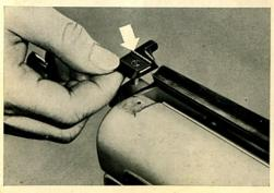
14/9 The holes for the trim panel clips are sealed with rubber caps. These rubber caps are used on the De Luxe Sedan for sealing the mouldings.
