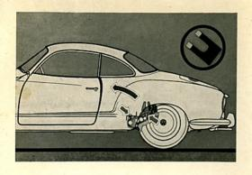
14/3 If this is not the case, the rear of the body must be raised until the gap between door and quarter panel is parallel.
