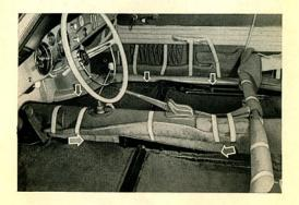
14/27 In order to observe the whole interior of the car during the spraying, the seats and floor mats should be removed and the carpeting turned up.
