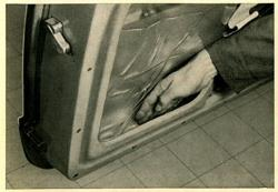
14/8 The plastic material inside the door directs the water to the door drain holes.
