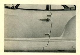
14/4 The door gap is now correct and will thus usually eliminate leaks at this location.
