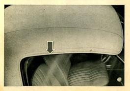
14/17 In this picture you see that the angled part of the weatherstrip is cemented horizontally at the hinge pillar. That is incorrect.
