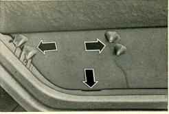
14/6 We remove the weatherstrip and the window glass. Two mechanics press the window channel together. The door must be pressed from the inside to avoid denting the door on the outside.
