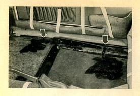
14/28 We start by spraying the weatherstrip between the body and the frame.
