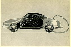
14/25 The previous pictures have shown us, that the difference in pressure or suction in the interior of the car strongly favours the entry of water whilst driving. If a customer complains of leaks, which you in your workshop cannot find by merely spraying the car, an attempt must be made to artificially create the difference in pressure obtained whilst driving.
