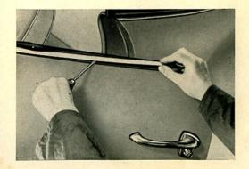
14/5 This weatherstrip is wavy and is not seated correctly on the glass. It must, therefore, be replaced. The removal and installation must be carried out carefully to prevent damage to the paintwork.
