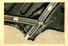
14/30 Now we nail the weatherstrip along the long side of the frame so that the end is gripped in the cutaway section of the front cross member weatherstrip, as indicated by the centre arrow on the right.
