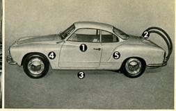
14/38 Next check the seams between the floor plates and frame tunnel. For this purpose the vehicle must be raised and a second mechanic equipped with a torch should watch the interior of the vehicle.
