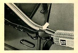
14/29 After we have raised the body we cut the front cross member weatherstrip to size and nail it in position. A section of the inner lip of this strip is cut out in order that the long weatherstrip around the frame, which is not shown in this picture, can be located in it. We put sealing compound on the long side of the frame immediately in front of the cutaway. The same operations are then carried out on the other side of the frame.
