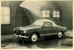
14/40 Now we turn to the upper portion of the body. For leaks at the rear side windows various points must be sprayed separately for about 5 minutes, in order to determine the actual location of the leak.
