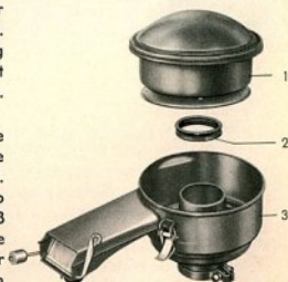
1 - Filter element, 2 - Gasket, 3 - Oil reservoir
