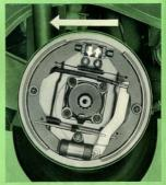
When adjusting the rear wheel brakes, the hand brake must be released. It is advisable to depress the brake pedal sharply before and after adjusting the brake shoes to ensure brake shoe centering, i.e. the proper position of the shoes relative to the brake drum.
