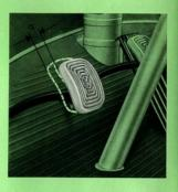
Measured at the clutch pedal this free play should be  $^1/_2$ " to  $^3/_4$ " (a). The clearance can be adjusted with the adjusting nut at the rear end of the cable.
