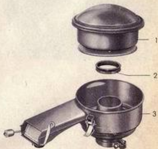
1 - Filter element, 2 - Gasket, 3 - Oil reservoir
