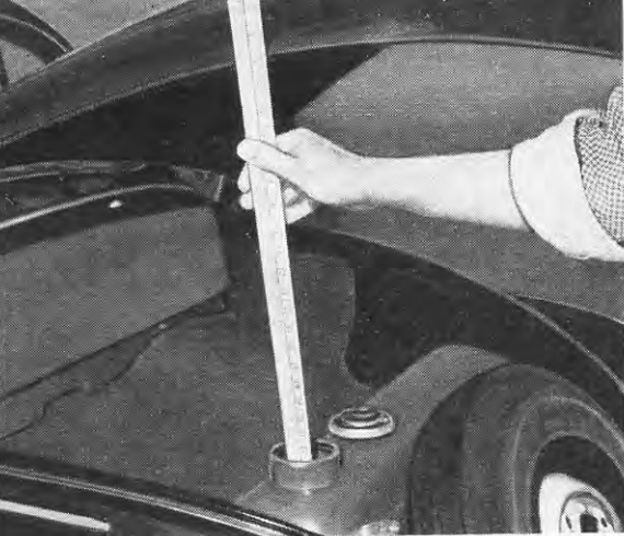
Above, the VW has no gas gauge. If you must know how much gas you have, use a yardstick! Below, some owners dislike the roller accelerator pedal (arrow)
