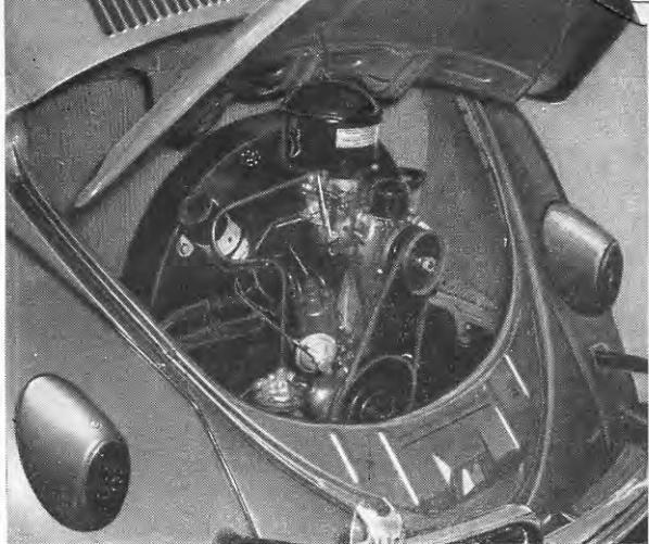
Above, air-cooled rear engine has only one fault, say owners: It’s a bit noisy. Below, the four cases fit inside car without infringing on seating space. One goes under hood, others pack behind rear seat
