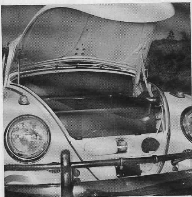
Front luggage space has been increased as a bonus from the re-designed gas tank. However, overall storage capacity is still comparatively limited.
