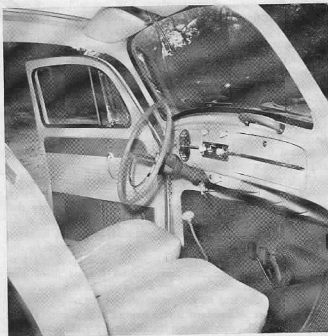
Few obvious changes have altered the appearance of the dash panel. One thing that is new, however, is the grab bar near the upper right panel.
