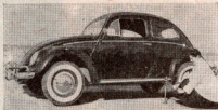
Slot in running board takes easy to work jack, raises entire side for tire changing.
