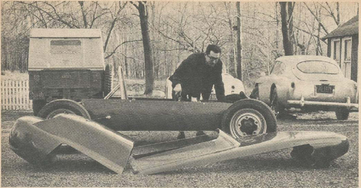
Ernie checks over the steering action before fastening on the top body panels. They are made of glass-reinforced polyster resin and can be ordered in a variety of colors.
