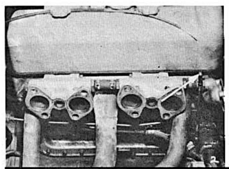
1-Remove flexible hose connecting air cleaner to air box on carburetor.
