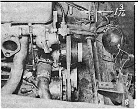
3—Install new crankshaft pulley making sure that the dowel extending from the crankshaft is inserted in the hole in the pulley. Use flat-washer next to pulley and internal lock-washer between head of bolt and flat-washer (use 74" Standard American socket). Reinstall original fan belt and obtain proper tension by tightening generator bracket. Place fan spacer on fan pulley hub as shown. Replace fan using four metric bolts furnished.
