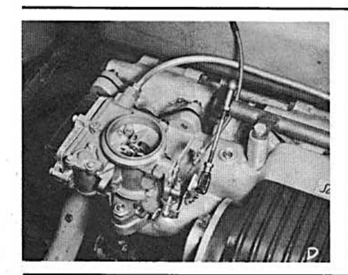
10—Fasten the carburetor to the supercharger as shown. Connect choke wire from control next to ignition key to carburetor choke (other choke control is not used and can be placed between lubricator and battery).
