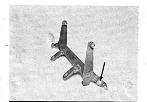
7—Remove the original throttle control from the carburetors. Remove lever arm which is fastened with set screw and reverse on shaft. (Both balls on end of arms now face in same direction.) Make sure that front and rear levers are in line and spot shaft with %" drill through the clamping bolt hole. This will permit the set screw to lock the arm to the shaft securely.
