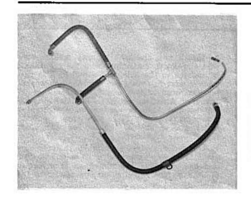
6—Cut off the end of original fuel line which was attached to the fuel pump. Retain original nut which will be used. Remove the insulation with bracket from tubing and slip over replacement fuel line. Bend new fuel line as shown in photo using the original fuel line as a guide or template.
