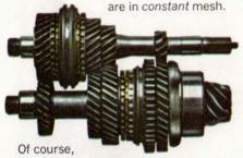
only one driving and one driven gear are actually locked to the shafts at a time. The three other sets of gears spin freely.
