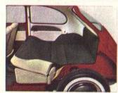
made the rear seat backrest collapsible. Just fold it down on the seat cushion.
