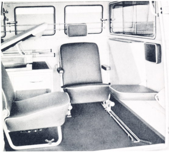
Stretcher folds back to accommodate second chair
